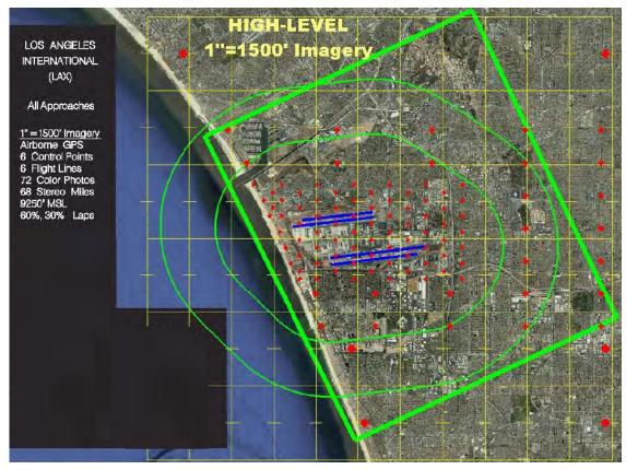
Figure 5. Coverage area for 1"=1500' photo scale (high-level)
