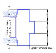
Figure 13. Door jamb - typical measure points
