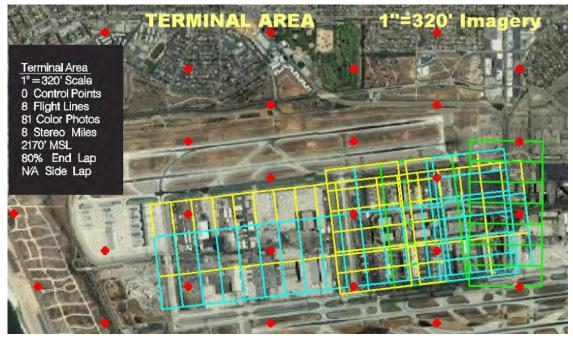
Figure 2. Terminal Area Model Limits
