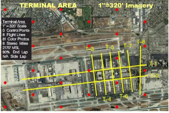
Figure 3. Terminal Area Flight line locations
