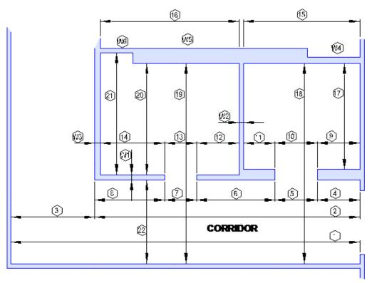
Figure 9. Wall thickness measurement guidelines
