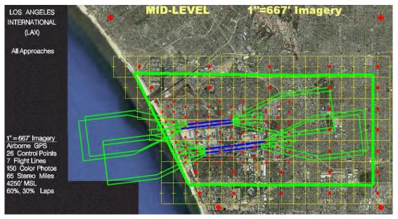
Figure 4. Coverage area for 1"=667' photo scale (mid-level)
