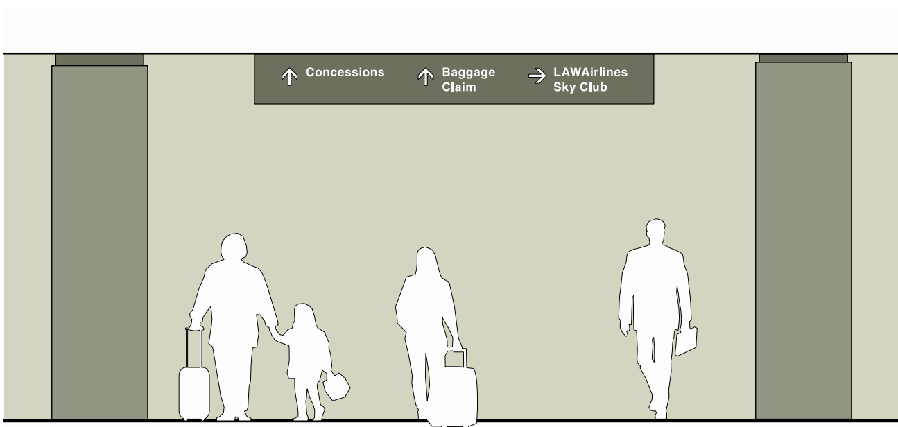
Figure 31: Directions to tenant passenger lounges may appear on airport directional signs by request to LAWA.
