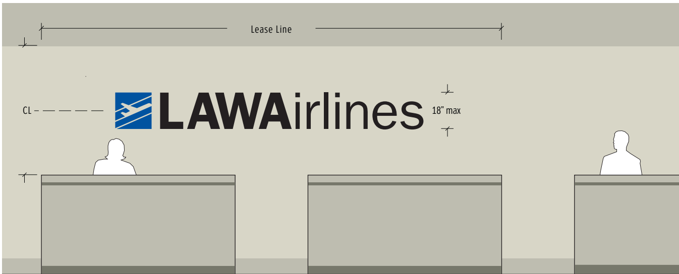
Figure 3c: Dimensional copy is the preferred treatment for corporate signature signs on walls behind ticket counters.
