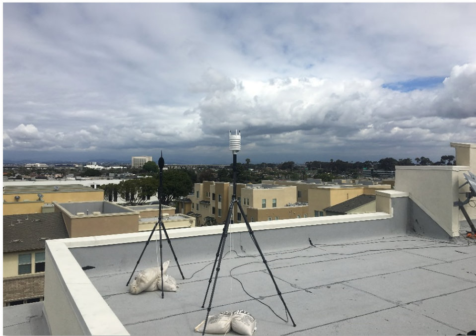
Figure 2-1. Photograph of Instrumentation Set-up (Sound Level Meter (left) and Weather Station (right)) at 360 Community, March 16, 2018, facing north towards LAX
