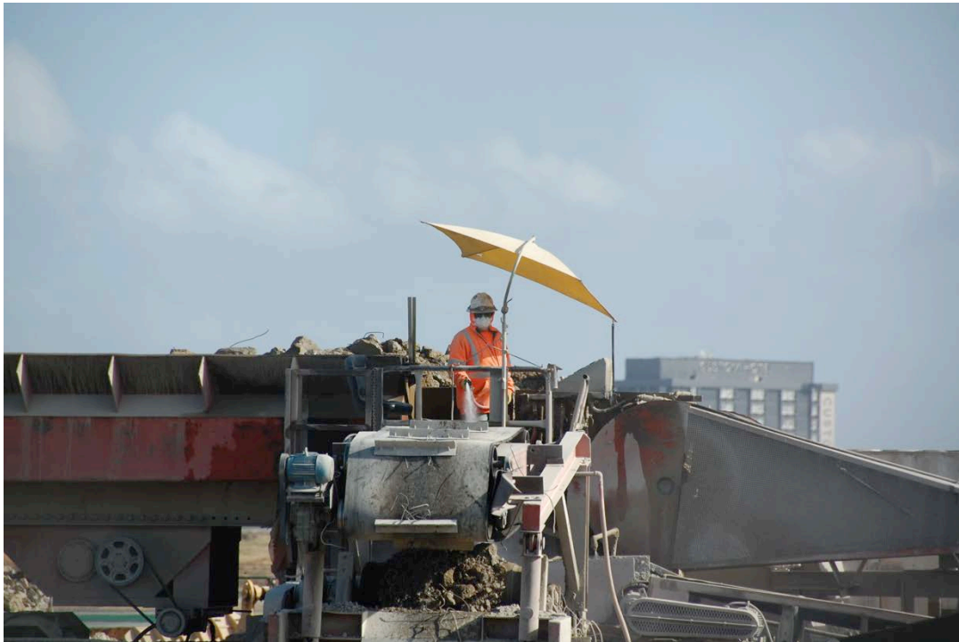
Figure 7-1: Fugitive Dust Control on the MSC Crusher
