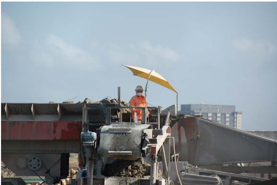
Figure 7-1: Fugitive Dust Control on the MSC Crusher
