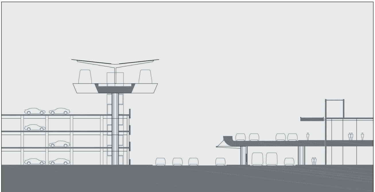
Figure 57 - APM garage-side option, in which passengers circulate down and across Arrivals roadway
