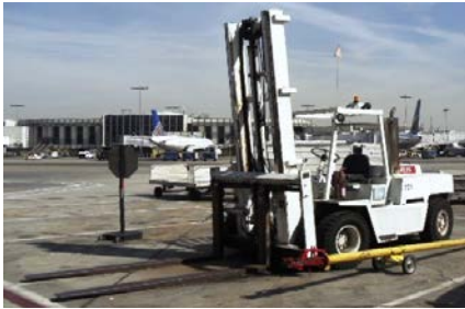
Current LAX GSE inventory includes emission-saving electric forklift
