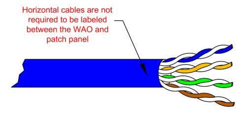
Horizontal copper cables between WAO's and patch panels are not required to be labeled.
