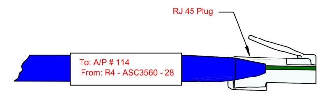
Horizontal cables with RJ 45 Plugs shall be labeled with origin and destination.
