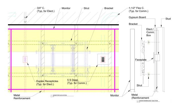
Sample CATV monitor installation layout diagram.
