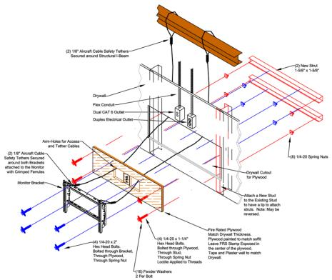
Sample single video monitor installation detail diagram.
