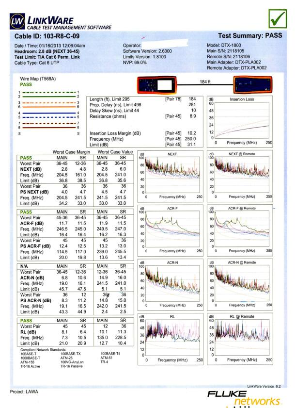
Sample CAT 6 horizontal cable permanent link test diagram.
