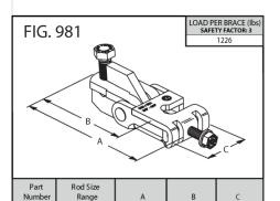
41/8" (104.8) 981-S 3/8" thru 5/8" 51/8" (130.2) 11/4" 51/8" (130.2) 41/8" (104.8) To Install: Slip the open side of the 981 yoke onto the all thread
