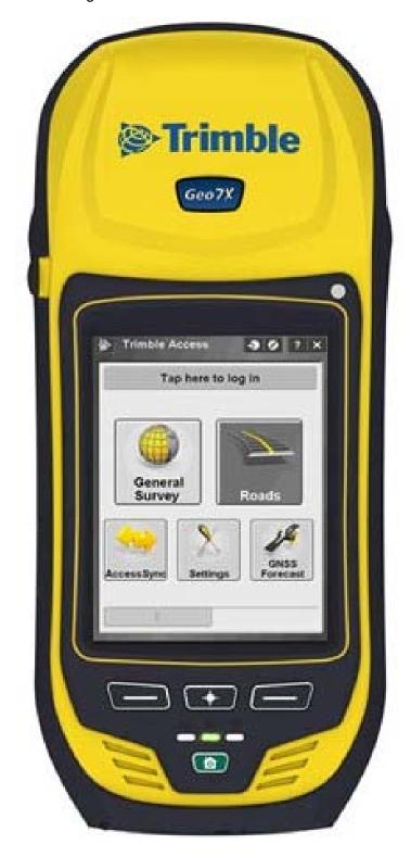
A Trimble Geo 7x GPS locator is pre-approved by LAWA for obtaining GPS coordinates.
