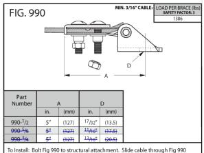
To Install: Bolt Fig 990 to structural attachment. Slide cable through Fig 990 and tighten break off nuts until shearing off. Attachment can pivot for adjustment to proper brace angle.
