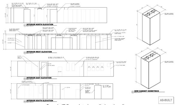
Sample IT Room interior wall elevation diagrams.
