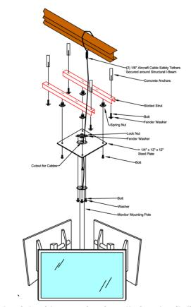
Sample triple video monitor installation detail diagram.
