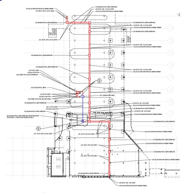
Sample conduit and junction box pathway diagram.
