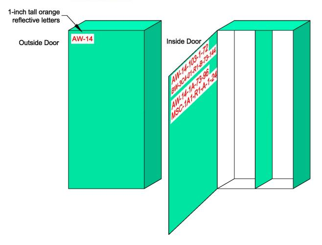
Patch Panel labels located on the outside and inside of panel.
