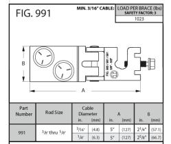
To Install: Slip the open side of the Fig 991 yoke onto the all thread rod above the top of the trapeze. Insert the cable through opening and out the back, pull tight. Tighten break-off nuts until nut shears. Secure in place with hex nut.
