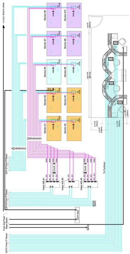
Sample Video wall wiring (interconnect) diagram.
