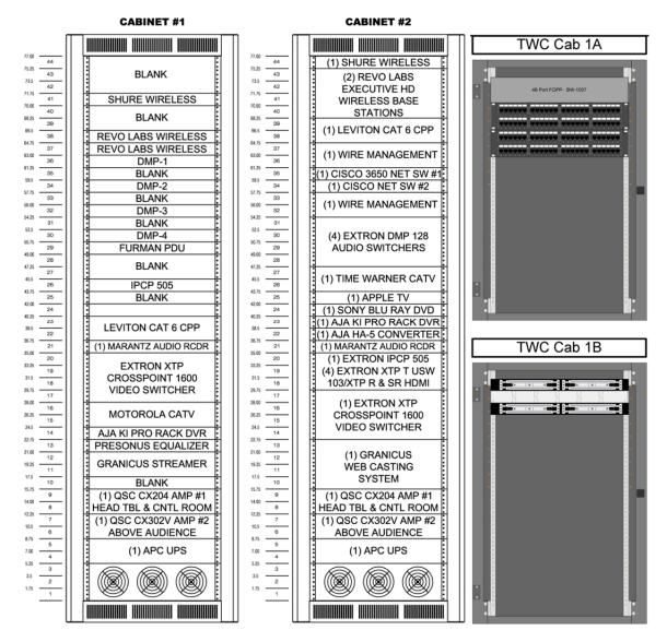
Sample equipment cabinet elevation diagrams.
