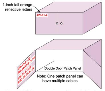
Patch Panel labels located on the outside and inside of panel.
