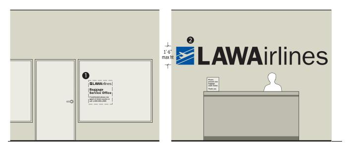
Figure 3j: An informational sign on the exterior window 1 and a corporate signature sign behind the service counter 2 inside the baggage service office.
