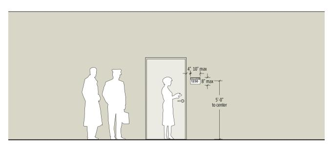
Figure 3n: Room identification signs which comply to ADA code standards are required by law.
