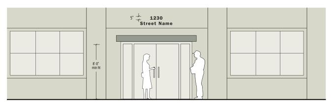
Figure 6a: Address size for a building set back 30' from the street (30'= 30" | 30"+10"=3" | 3"+2"=5").
