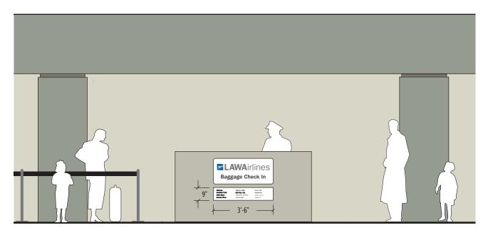
Figure 3o: Airline alliance identity sign on the baggage check-in counter.
