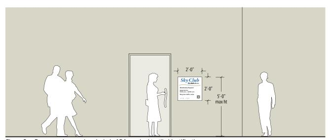
Figure 3m: Passenger lounge signs include ADA required tactile identification.
