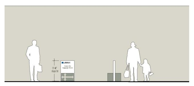
Figure 3g: Standard luggage sizers minimize clutter in the terminal.
