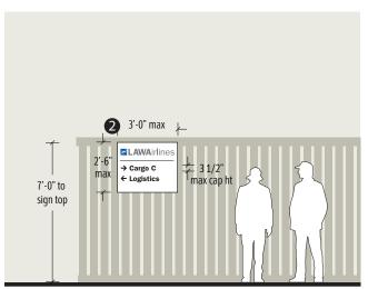
Figure 6d: Directional signs guide vehicular traffic to tenant buildings when other such signs do not exist.
