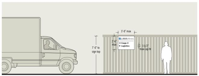
Figure 6c: Fence signs are permitted but not desired.
