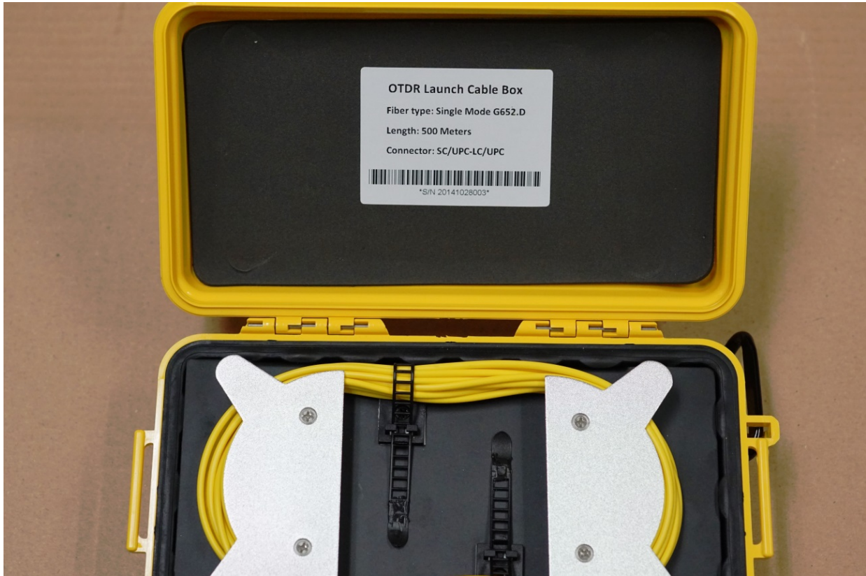
A professional fiber optic launch box is required when using OTDR's.
