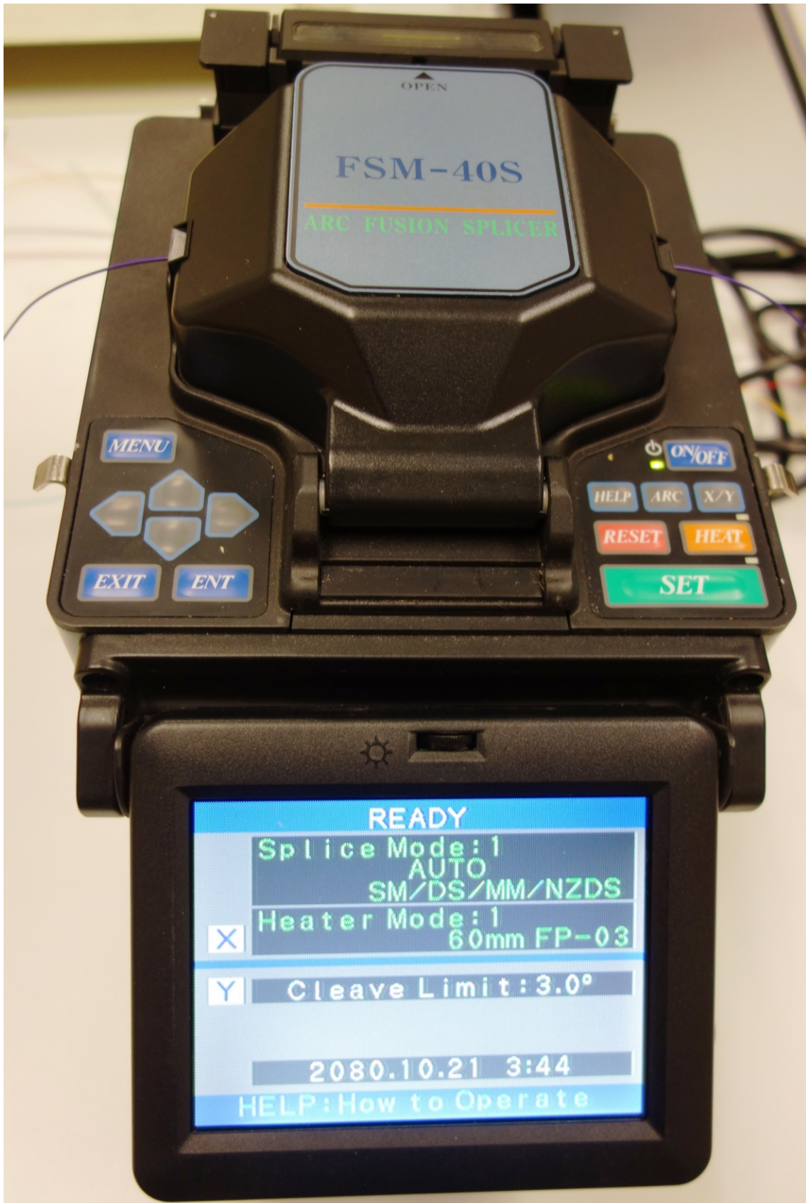
A fiber optic fusion splicer is required joining fiber strands, and older model is shown.
