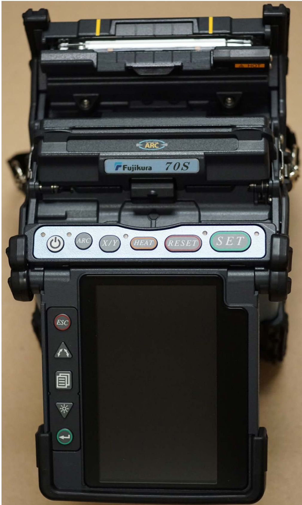
A fiber optic fusion splicer is required joining fiber strands, and newer model is shown.
