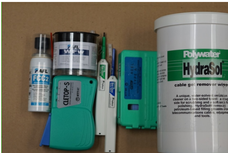
Fiber optic cleaning supplies are required to be used with test equipment.
