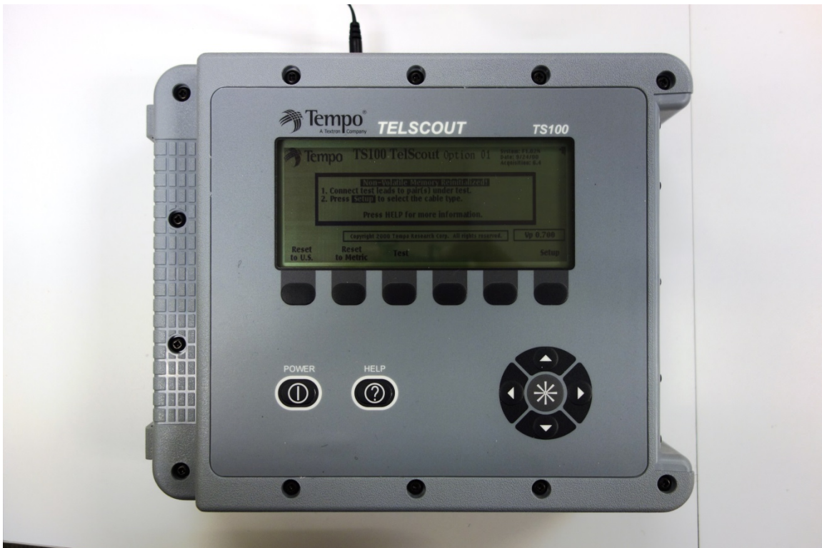
T-1 circuit tester for testing and troubleshooting.
