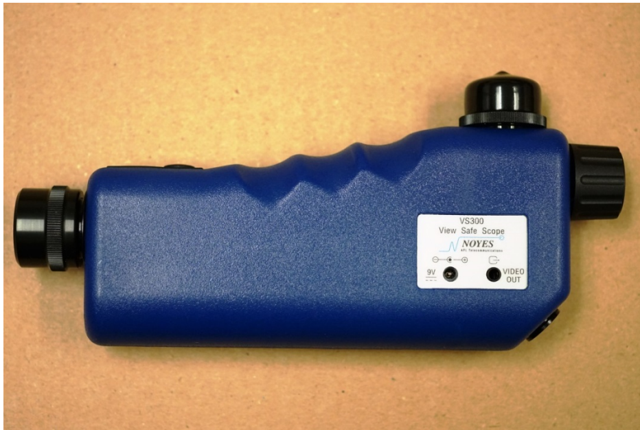
A 400x fiber microscope is required to examine singlemode fiber.
