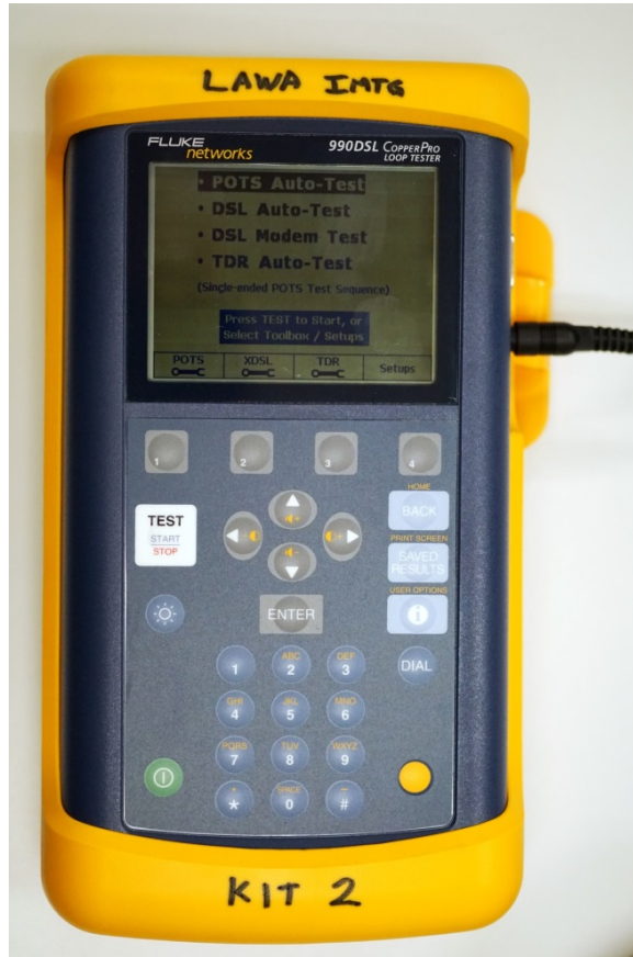
DSL circuit tester for troubleshooting.
