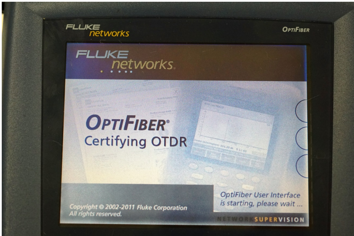
An Optical Time Domain Reflectometer is required to test, certify, and troubleshoot fibers.
