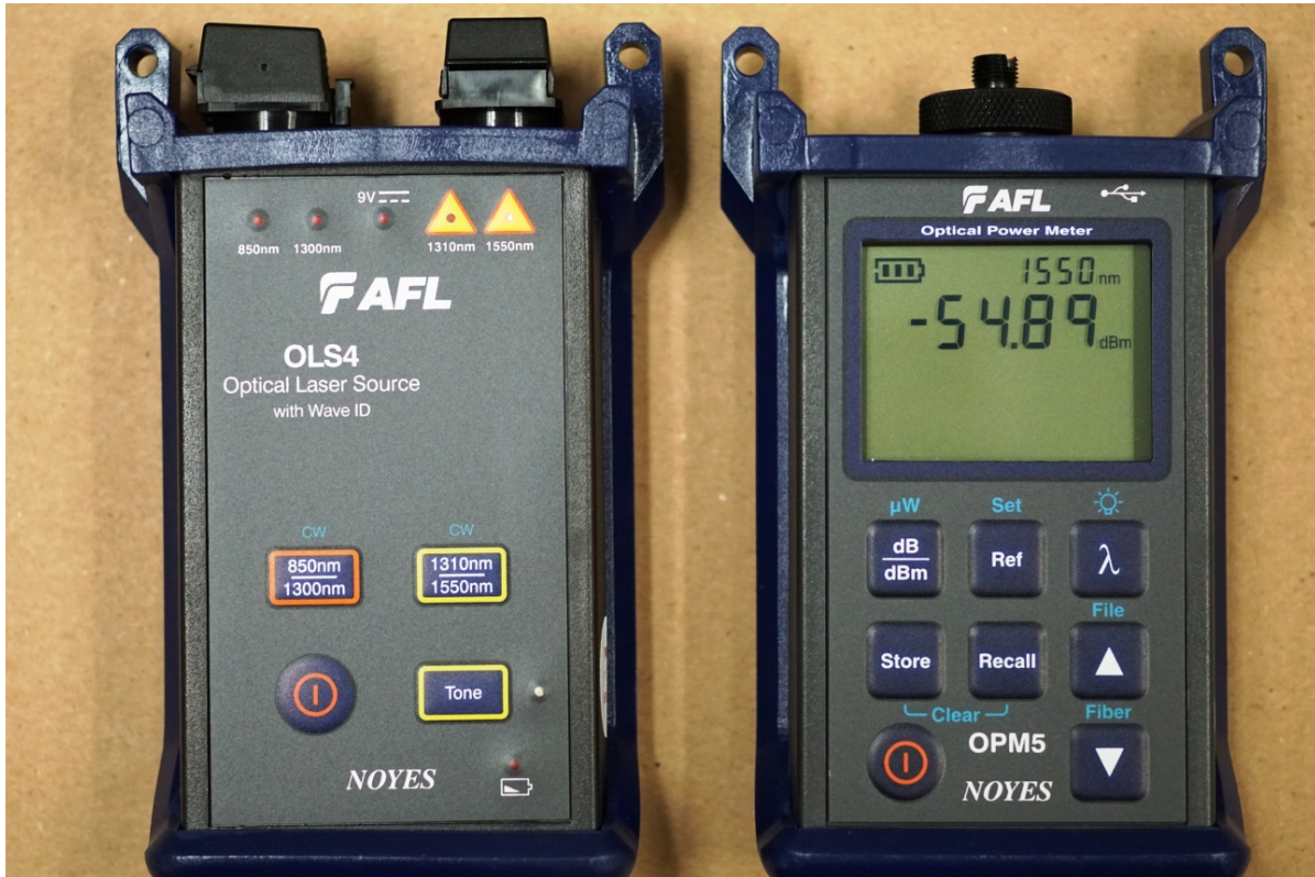
A Fiber optic light source and power meter is required for obtaining accurate signal loss levels.
