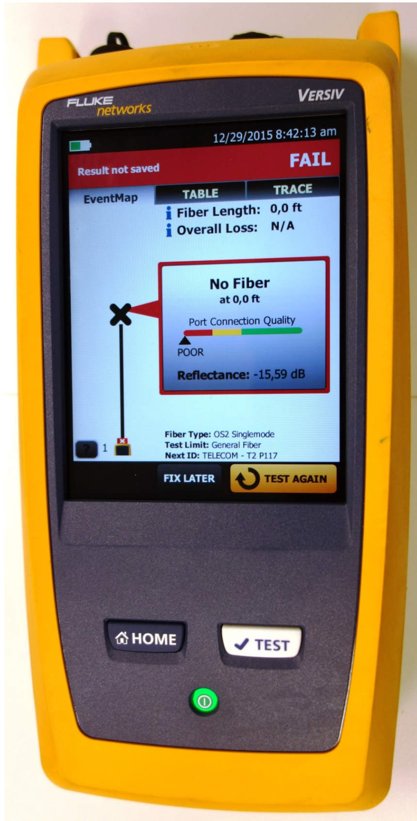
An Optical Time Domain Reflectometer is required to troubleshoot fibers.
