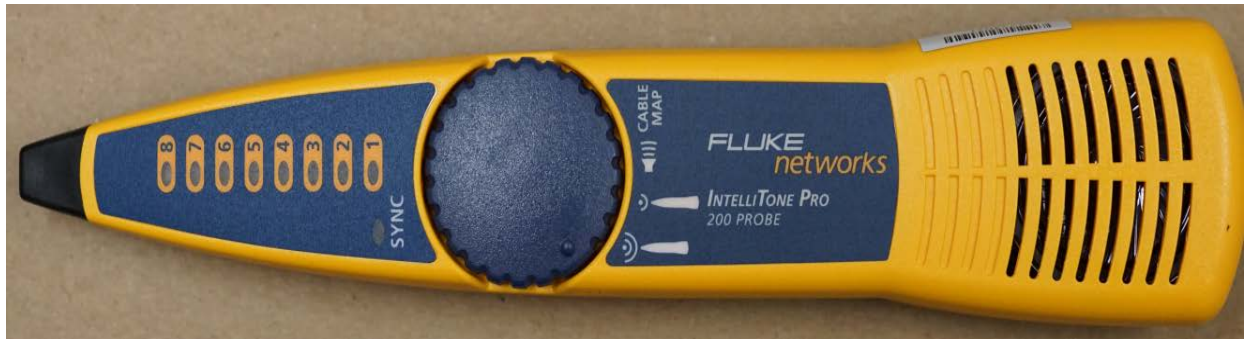
Tone generator and probe are used for identifying and troubleshooting copper.
