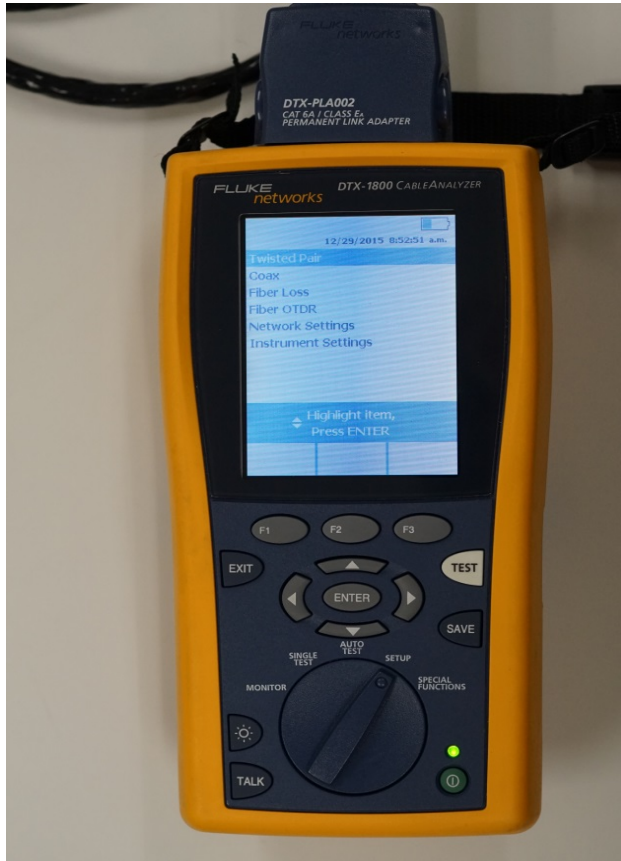
CAT 6/6A tester required for testing and certifying cable installations.
