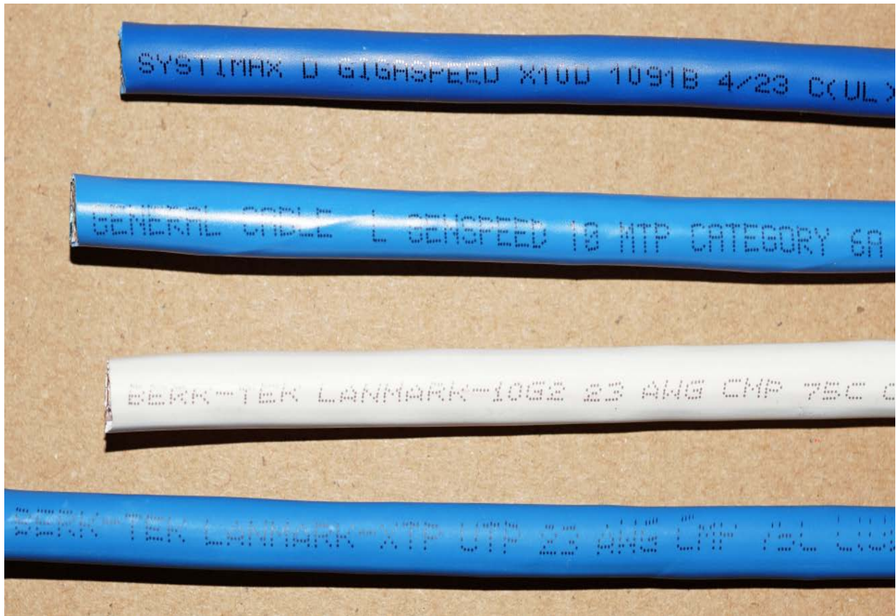
Legacy CAT 6A cables shown.
