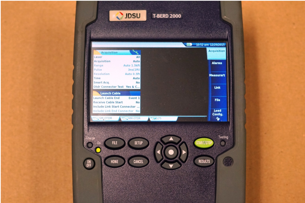
An Optical Time Domain Reflectometer is required to troubleshoot fibers.
