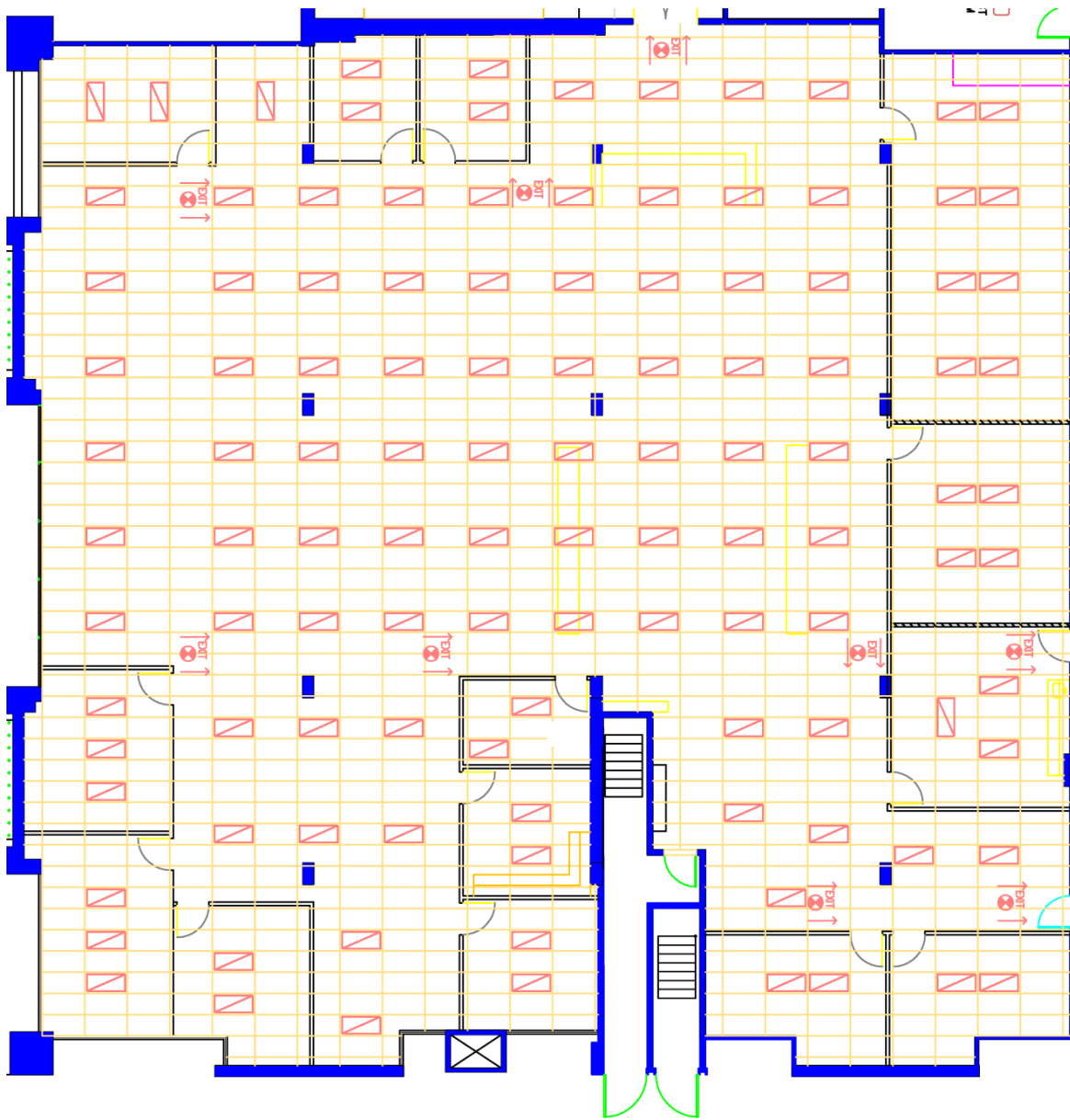
Sample Reflected ceiling diagram showing light fixture placement.
