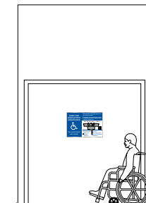
M_8 AREA OF ASSISTANCE SIGN
