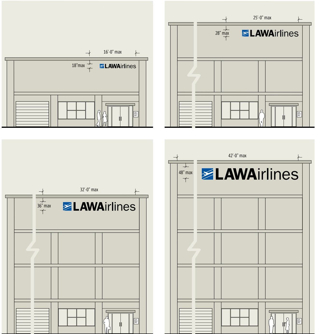
Figure 4c: Building height and width determine the maximum sign size for corporate signatures.
