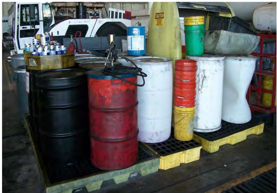
Photograph 52: View of hazardous waste storage area containing waste oil and aircraft hydraulic fluid.
