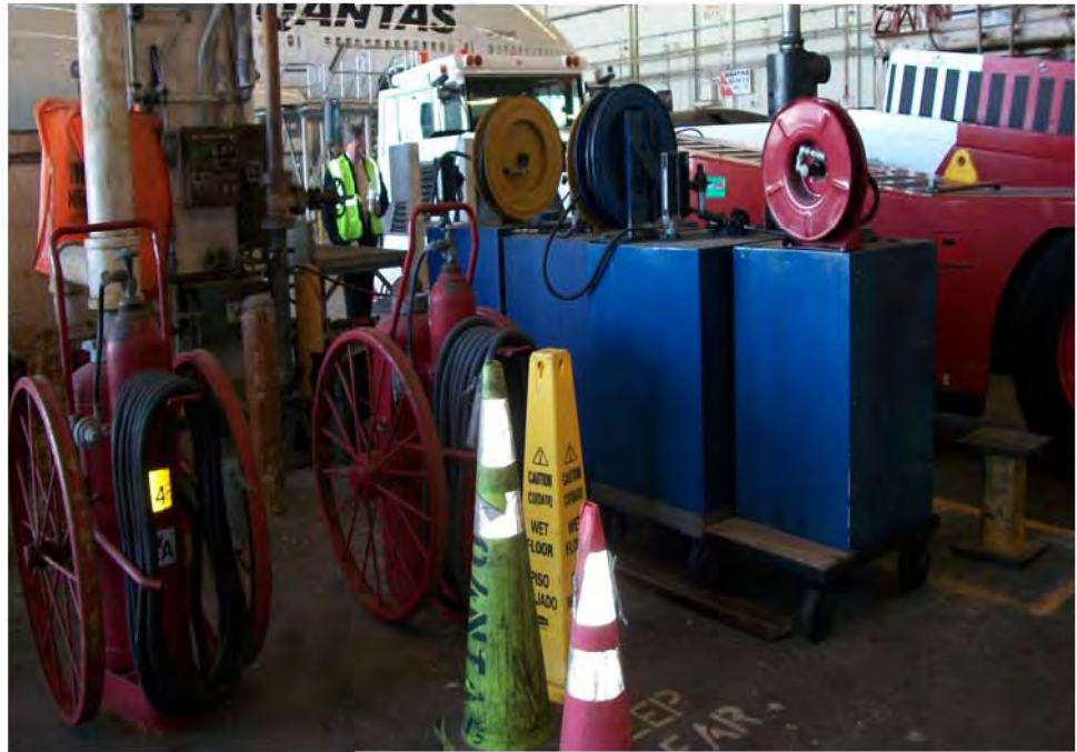
Photograph 51: View of one 75-gallon gear oil mobile AST and three 120-gallon hydraulic fluid, transmission fluid, and degreaser mobile ASTs in the central western portion of the Qantas hangar.
