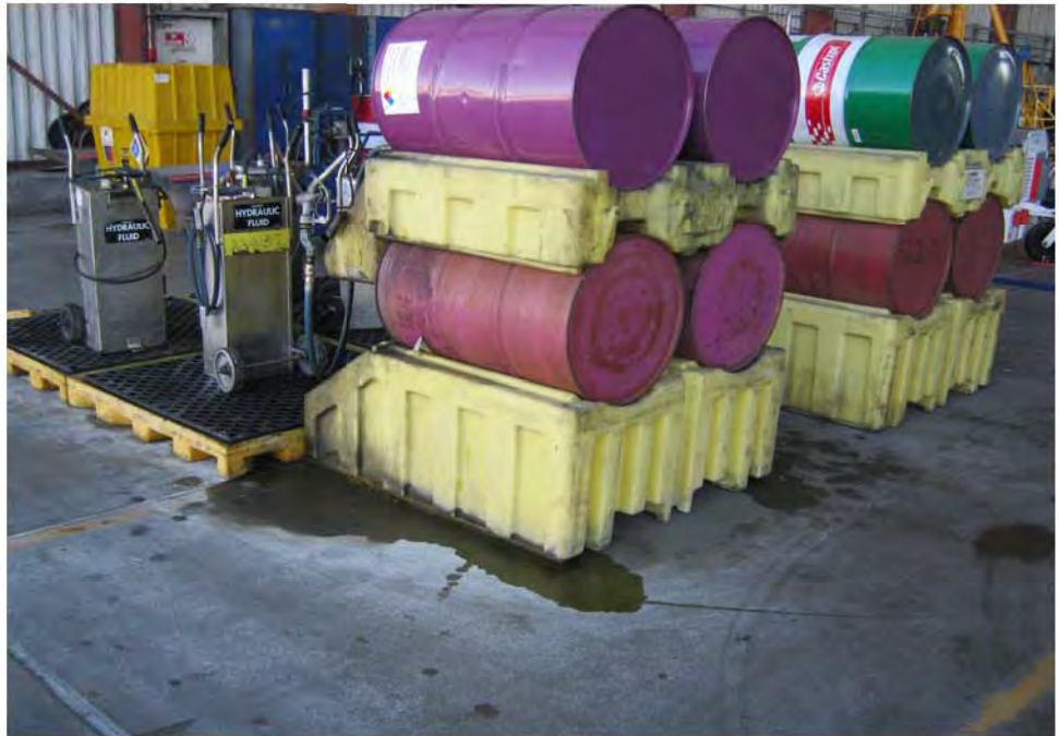
Photograph 97: View of hydraulic fluid staging area with pavement staining in the northeastern portion of the American Airlines hangar.
